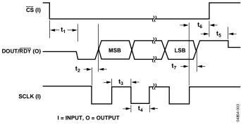
Figure 3. Read Cycle Timing Diagram
