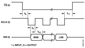
Figure 4. Write Cycle Timing Diagram
