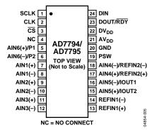
Figure 5. Pin Configuration
