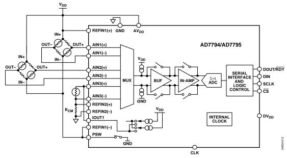
Figure 12. Basic Connection Diagram
