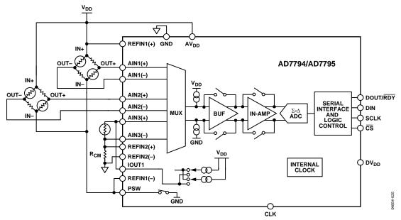
Figure 24. Typical Application (Flowmeter)
